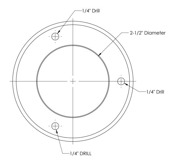
Please print at 100 percent for accurate sizing. Slight scaling may still occur. Therefore, before drilling, it is recommended that all template dimensions be measured for accuracy.
